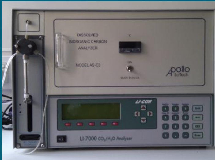
Front view of the DIC Analyser (Apollo SciTech) in use at NOC, Southampton (left); Total Alkalinity Titrator system (Apollo SciTech; right)
