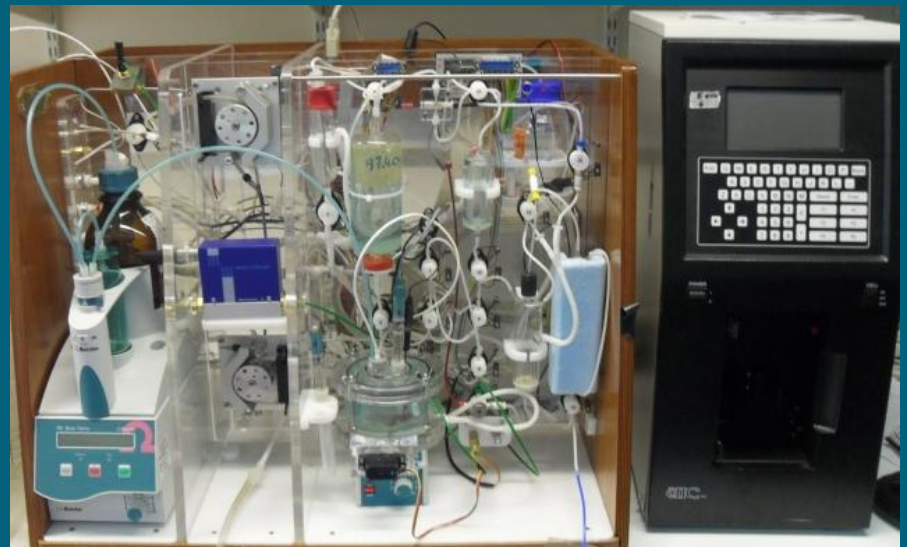
Front view of the VINDTA 3C and the UIC coulometer in use at NOC, Southampton
