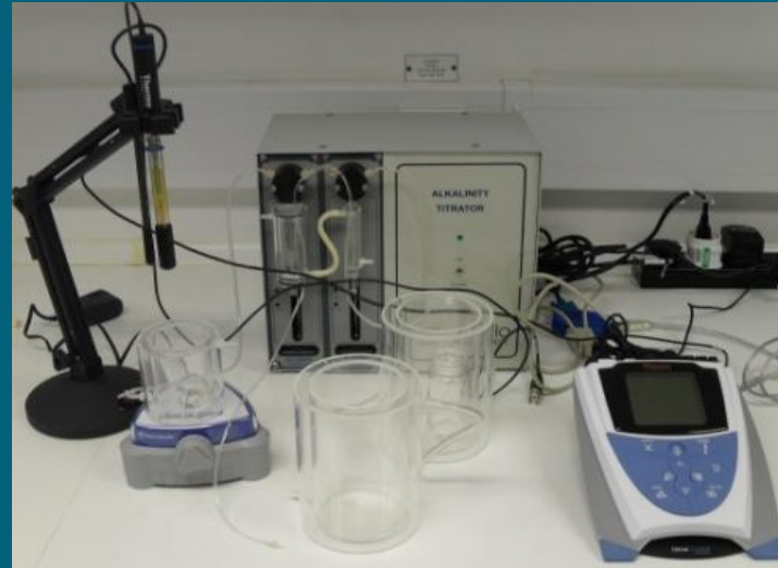
Front view of the DIC Analyser (Apollo SciTech) in use at NOC, Southampton (left); Total Alkalinity Titrator system (Apollo SciTech; right)
