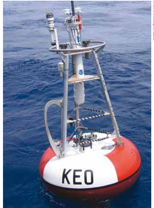
A NOAA mooring in the Pacific used to measure CO 2 fluxes.
