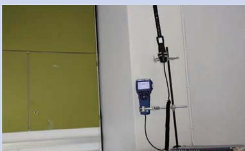
Figure 1: The CO<sub>2</sub> sensor is mounted on a stand and held with a clamp on a cupboard at the back of the classroom. This way the pupils are not distracted. Ensure free air circulation around the sensor.
