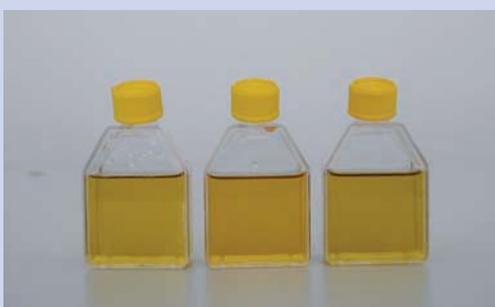
Figure 2: CO<sub>2</sub> was added by blowing air into the bottles. The yellow colour indicates that the water became more acidic.
